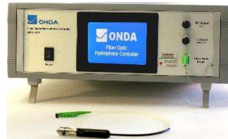
Fibre optic hydrophone
